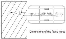
Please choose the suitable wall firstly. Fix M5 screw on the wall with distance of 60mm
